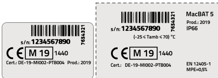
Figure 9. Nameplate placed on front door of the device (left – plastic housing, right – metal housing)
