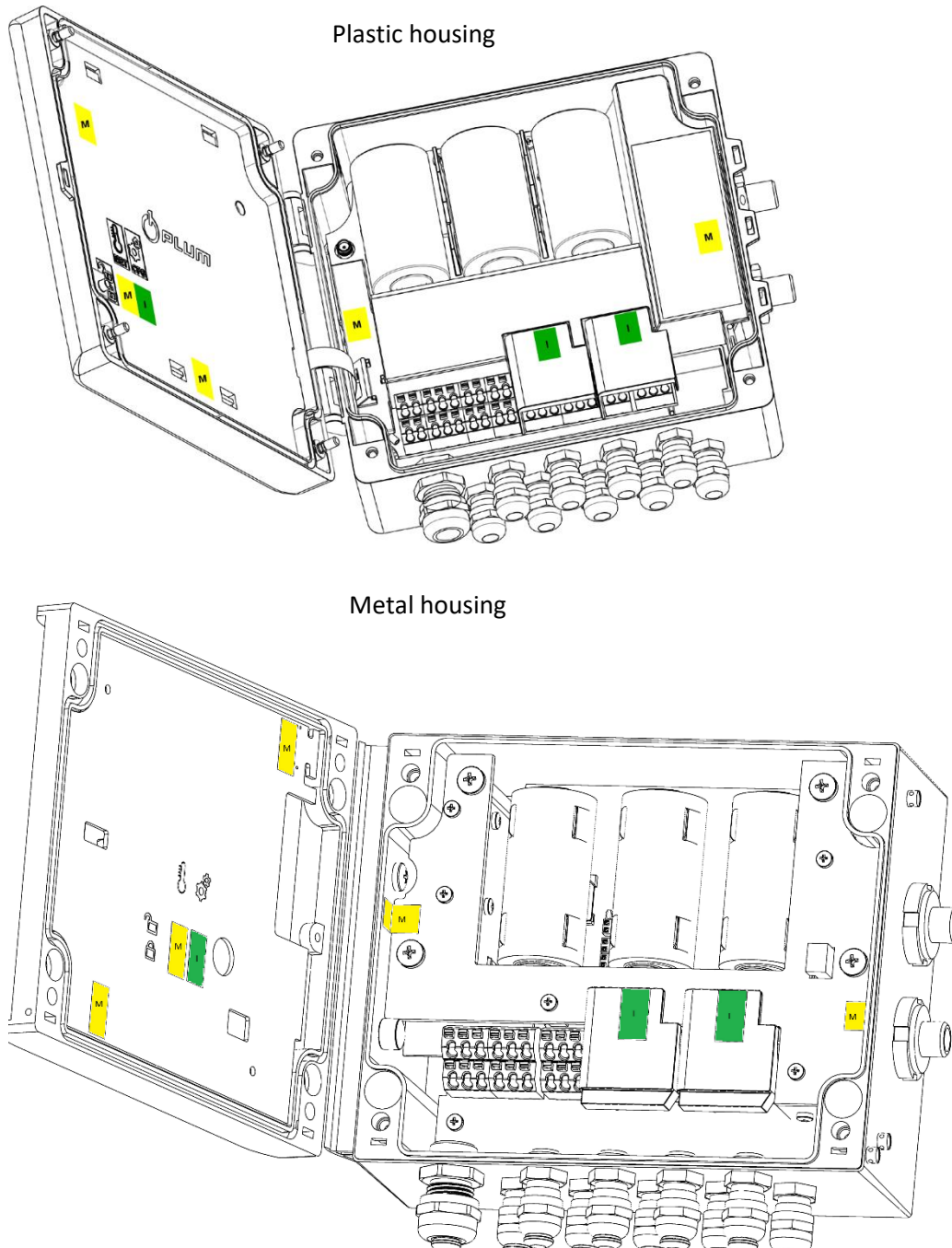
Figure 6. Internal sealing of MacBAT 5
